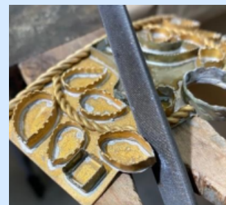
filing the edges after soldering
