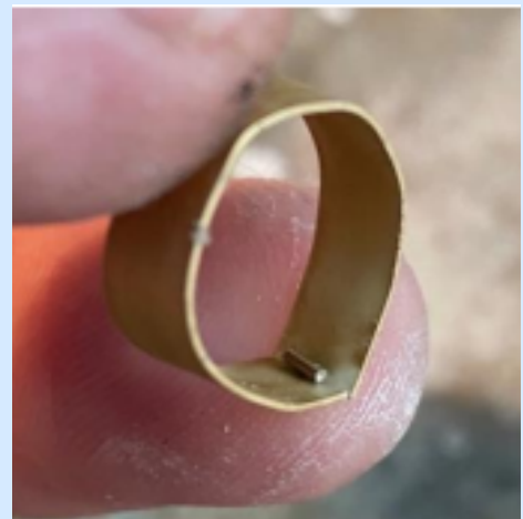
a piece of solder at the joint
