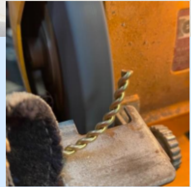
grinding the backs flat
